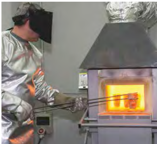
Smelter analysis in the MATSA mine laboratory, Seville, Spain.
